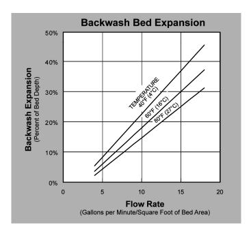
**BACKWASH** — After each cycle the media bed should be backwashed at a rate that expands the bed 20 to 40 percent.
